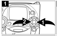
After you insert the disc into the CD player and the total number of tracks appear on the display, you may press either the Skip/Search ( $\succ$ ) ① or ( $\bowtie$ ) ② button to select a specific track for playback.
